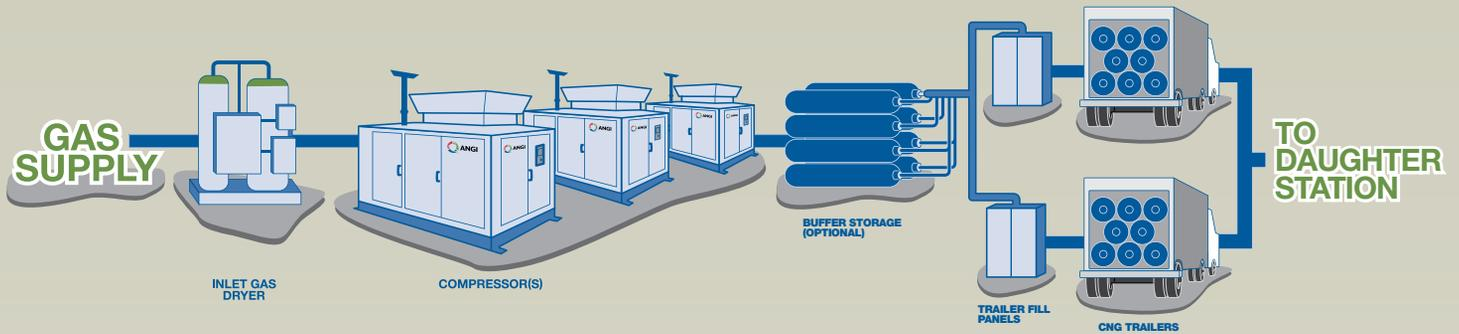
**DAUGHTER SYSTEMS** are installed where a CNG fill station utilizes mobile CNG storage as the fuel source for the station.
