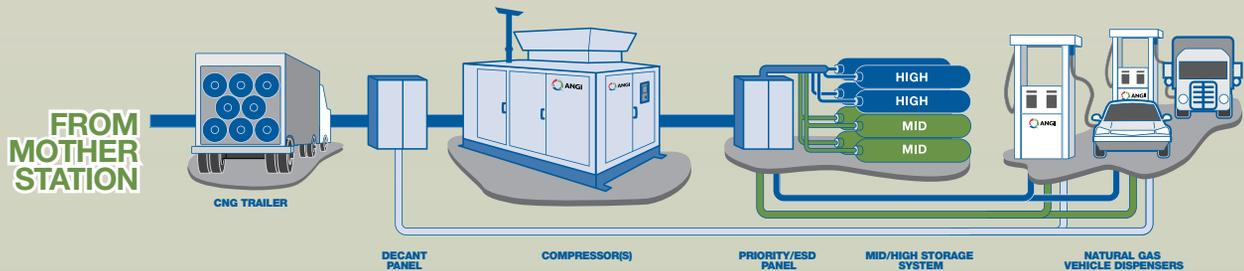
**TUBE TRAILER SYSTEMS** are used to supply industrial operations and stationary engines with natural gas where there is no natural gas pipeline.
