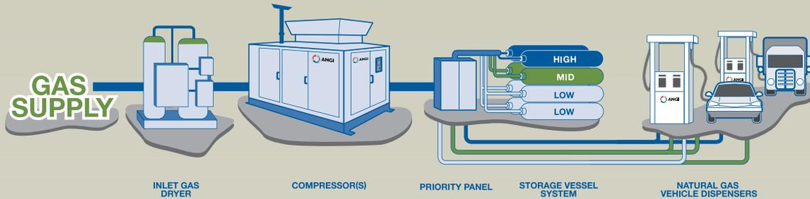
**TIME FILL SYSTEMS** are a cost effective fueling option that allow vehicles to conveniently refuel overnight or when the vehicles are not in use.
